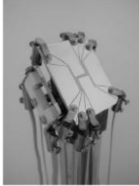
Figure 5: Photograph of the atom chip. The electrical connections via the copper tabs are visible on the four corners of the chips. The rubidium dispenser can be seen on the left side of the chip mount.
